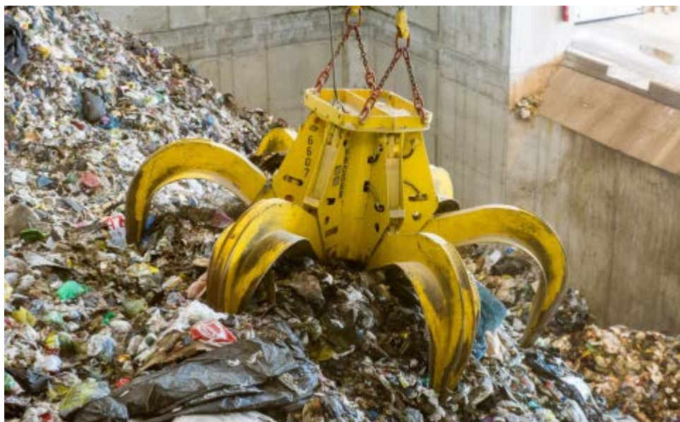
Figure 25 – Photo of a grab crane in action in a waste bunker (Kamuk, 2013)
